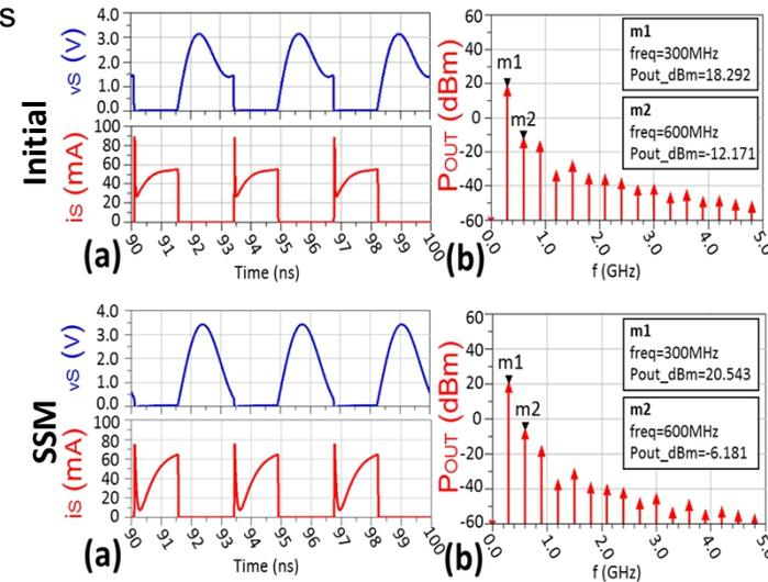
(a) **Simulated** Time domain waveforms: on the left, at the top the switch voltage,  $v_s$ , below, the current,  $i_s$ . (b) On the right the FFT of the  $P_{OUT}$ .
