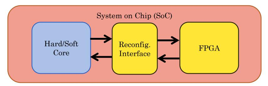
DPR allows the Core to load inside the FPGA the required hardware module only when it is necessary.
