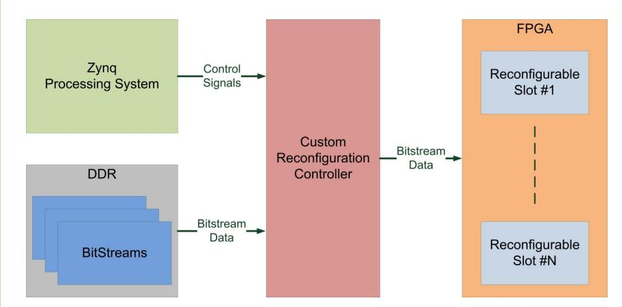
• Zynq Processing System can trigger a hardware reconfiguration by sending the bitstream to configure to the Reconfiguration Controller.
