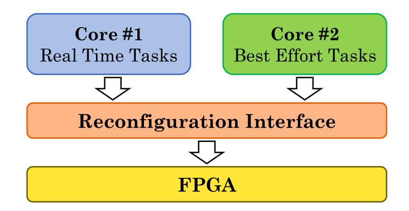
Both RT tasks and BE tasks can trigger a hardware reconfiguration. The reconfiguration interface will be a shared resource between the two cores and among all tasks.
