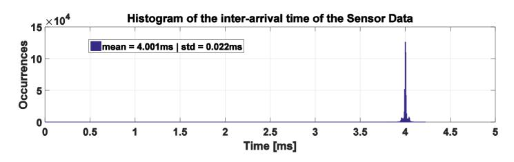
Precise and accurate triggering of the board
