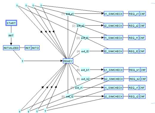
Invocation of a custom Java module for simulation at each event trigger
